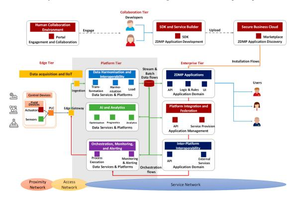
**Figure 10.** Mapping of Zero Defect Manufacturing Platform (ZDMP) high level architecture to the four tier architecture pattern.
