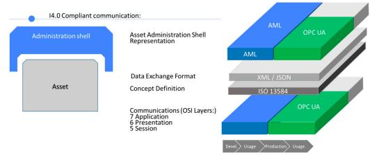
Figure 2. I4.0 Communication protocol stack.
