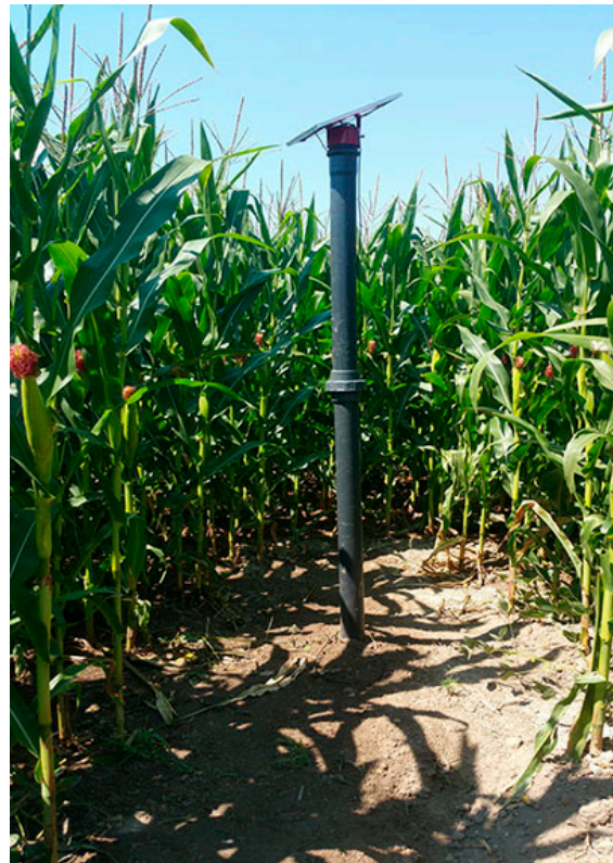
Figure 14. Environmental and soil wireless sensor deployed in the “Kopaida” farm maize parcel.
