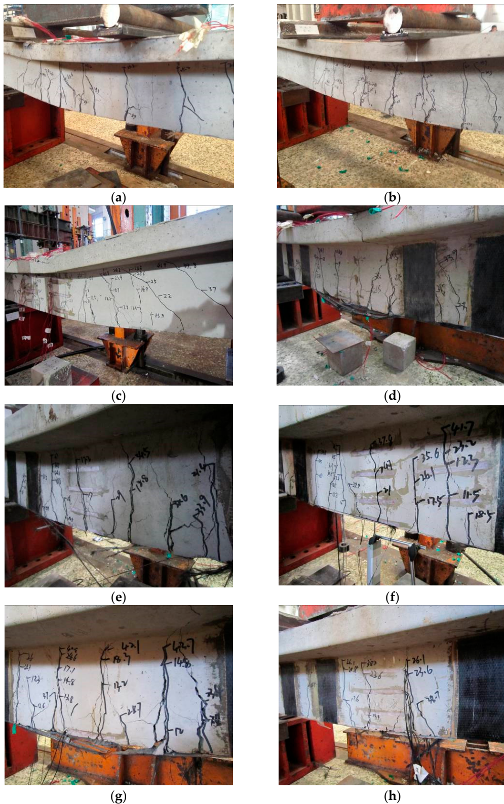
Figure 5. Cracks developed in RC T-section beams strengthened by CFRP. (a) B1 (b) B2. (c) B3 (d) C1. (e) C2 (f) C3. (g) C4 (h) C5.
