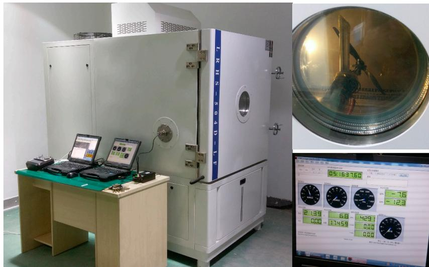
**Figure 3.** The discharge test of energy system in low-temperature and low-pressure test chamber.
