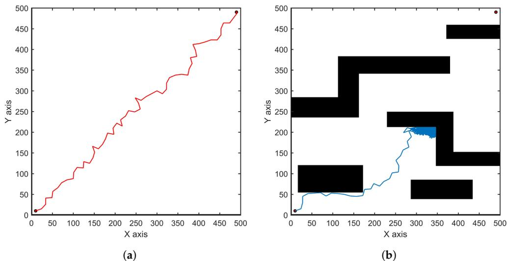
**Figure 3.** Under a *control* value of one and the combination of the exploration with the CSA method, the random tree exhibits different behaviors when it does and does not encounter obstacles. (a) Efficient exploration in an environment without obstacles. (b) The “local trap” phenomenon during exploration in an environment full of obstacles.
