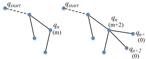
**Figure 2.** The change strategy of node state value  $\delta$  in the node control mechanism.  $q_{start}$  is the initial node, and  $q_n$  is any node in the tree.  $q_{n+1}$  and  $q_{n+2}$  are child nodes of  $q_n$ . The values in parentheses are the node state values  $\delta$  we recorded.
