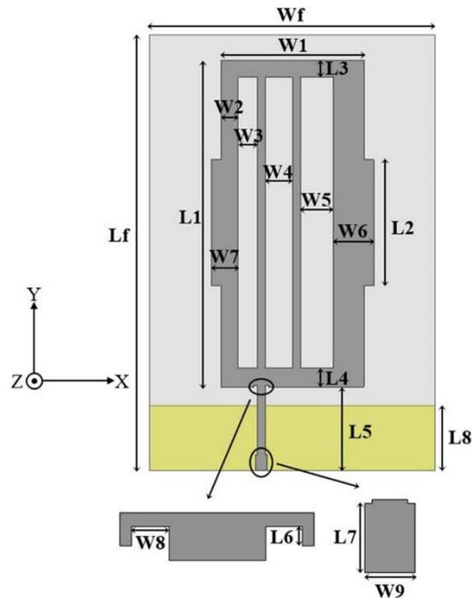
Figure 8. The geometry of the proposed UHF antenna.
