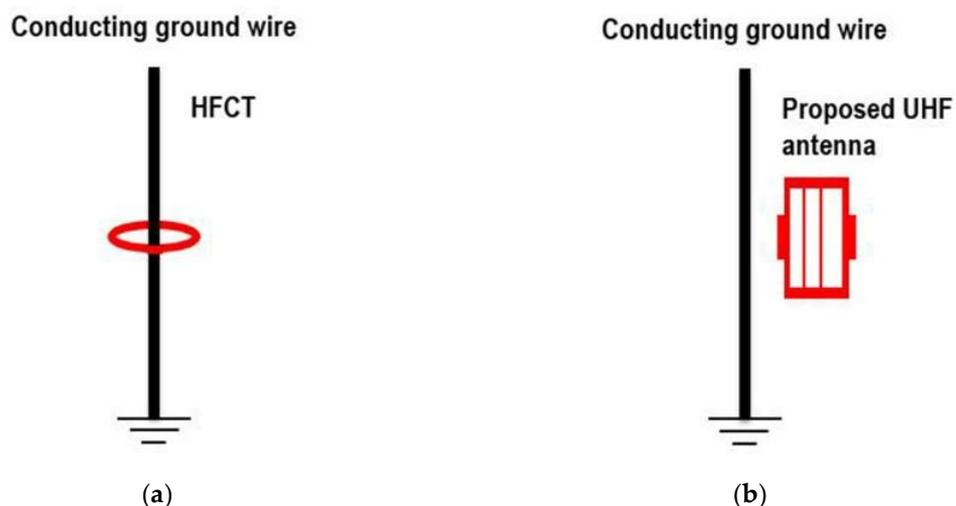
**Figure 2.** Conceptual diagram for the PD detection in the conducting ground wire: (a) HFCT and (b) proposed ultra-high frequency (UHF) antenna.
