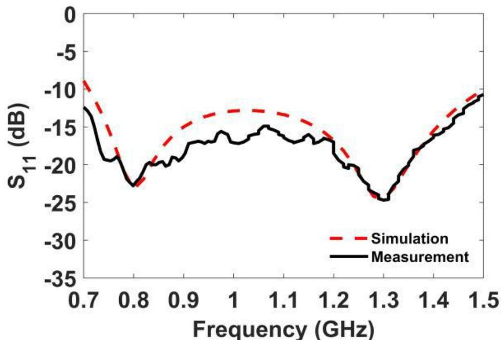
Figure 11. Simulation and measurement results ( $S_{11}$ ) of the proposed UHF antenna.
