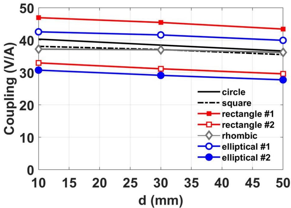
Figure 4. Coupling performance of each antenna.
