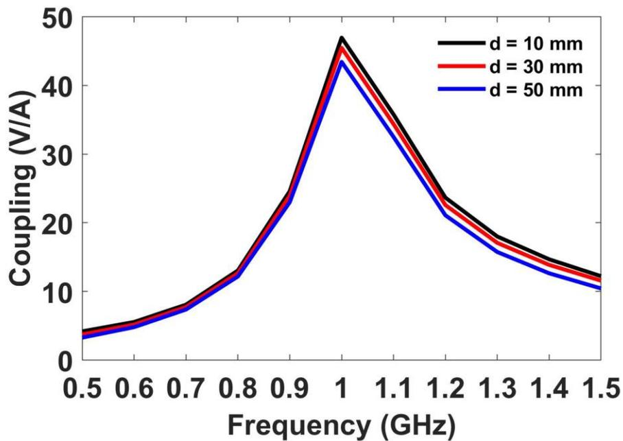
Figure 5. Coupling performance by rectangle #1 versus frequency.
