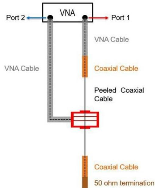
**Figure 12.** PD experimental set-up for the antenna test.
