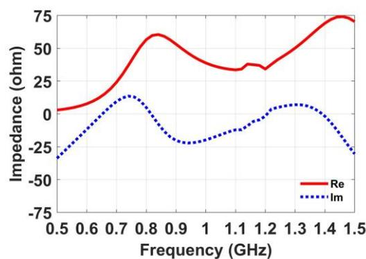
Figure 9. Input impedance of the proposed UHF antenna.
