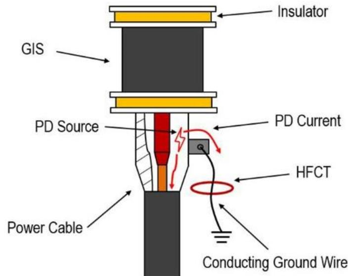
**Figure 1.** Partial discharge (PD) detection mechanism using the high-frequency current transformer (HFCT).
