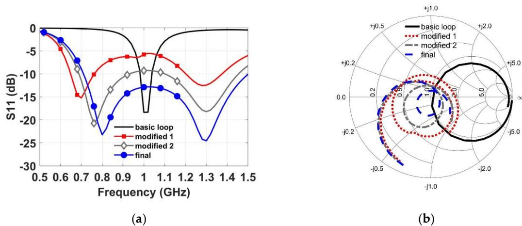
Figure 7. Antenna matching performance: (a)  $S_{11}$  parameters. (b) Smith chart.
