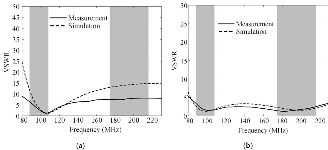
Figure 5. Impedance matching characteristics of the proposed antenna: (a) conventional thin dipole; (b) proposed antenna.
