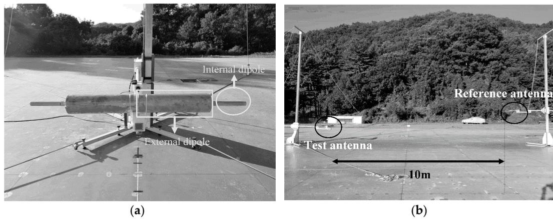
Figure 4. Outdoor test site: (a) antenna under testing; (b) outdoor test configuration.
