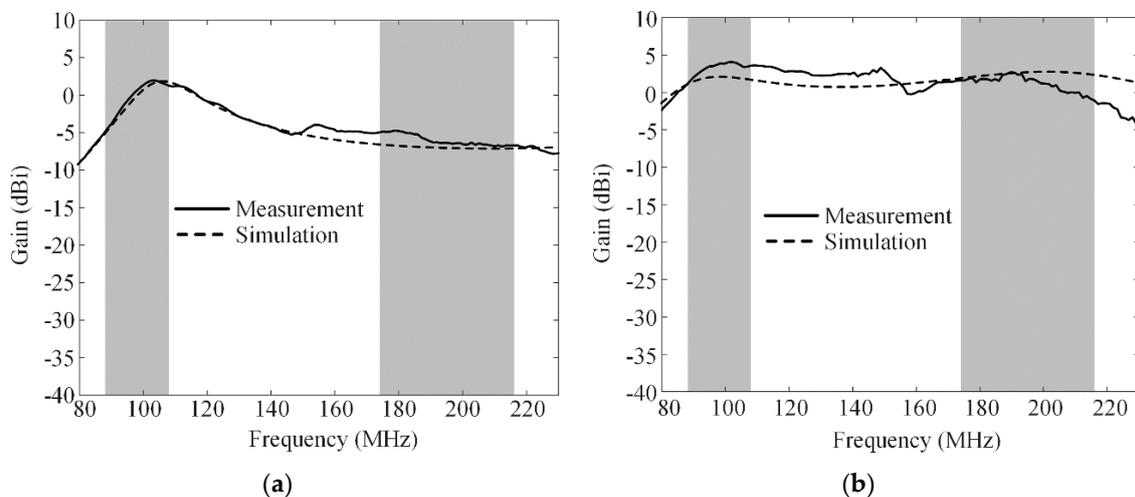
Figure 6. Bore-sight gains: (a) conventional thin dipole; (b) proposed antenna.
