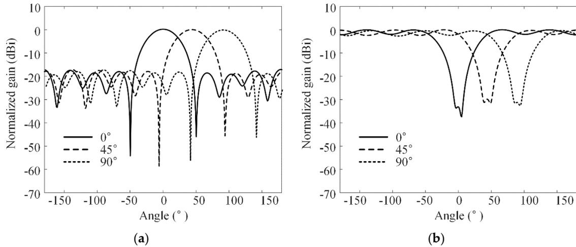
Figure 8. Optimized radiation patterns: (a) reference channel; (b) surveillance channel.
