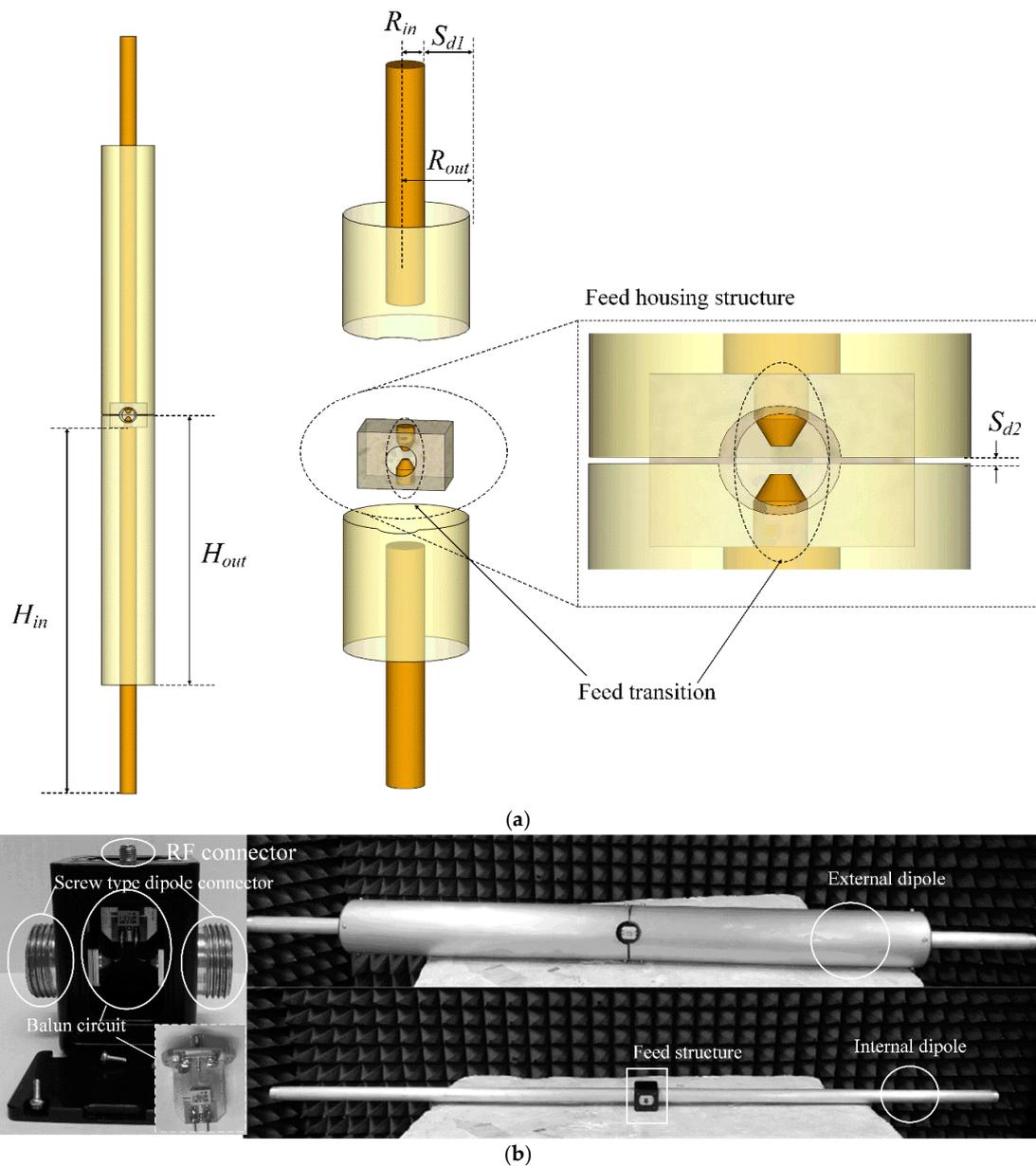
**Figure 3.** Geometry of the proposed antenna; (a) designed structure; (b) photographs of the fabricated antenna.
