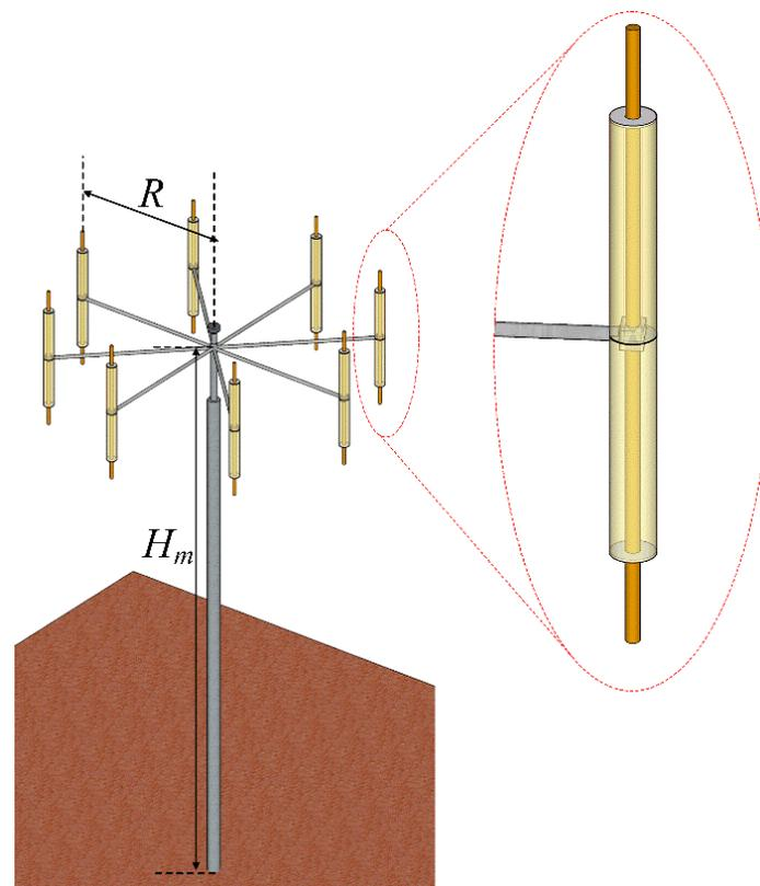
Figure 7. Array configuration of the PCL system.
