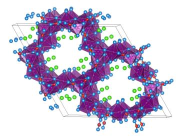
**Figure 5.** Crystal structure of the chlorartinite phase. Color scheme is the same as in Figure 1; carbon atoms located in the centers of triangular carbonate molecules are in red.
