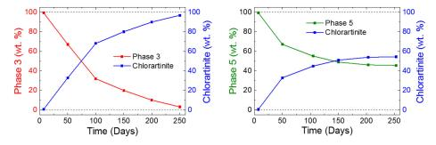
**Figure 6.** Phase composition of the surface of Phases 3 and 5 after 7, 50, 100, 150, 200, and 250 days of samples ageing.
