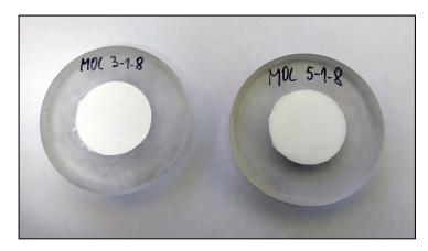
Figure 2. Photography of prepared samples in XRD holders: Phase 3 (left) and Phase 5 (right).
