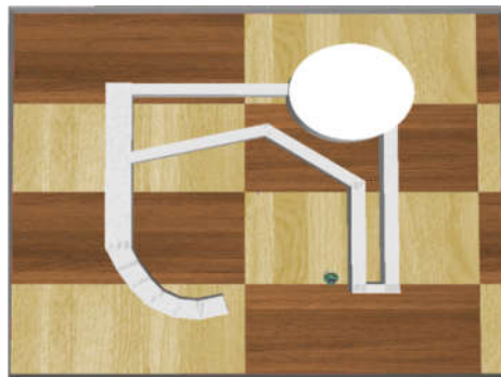
Figure 17. Training setting for wall-following control.
