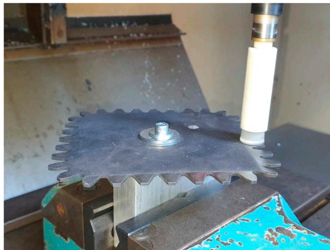
Figure 17. Deburring of a non-circular gear with rotary brushes with ceramic fibers.
