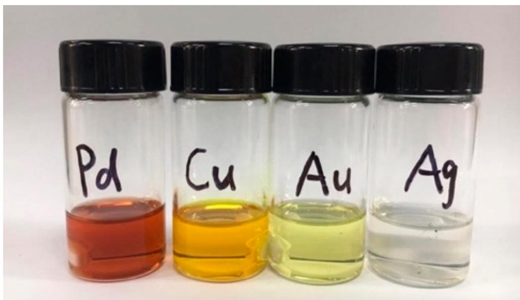
**Figure 1.** Metals dissolved by trichloroisocyanuric acid (TCCA)/ $N_{4441}Cl$  (the dissolved metals are Pd, Cu, Au, Ag from left to right, respectively).
