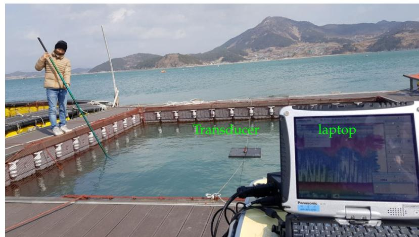
**Figure 2.** An experiment performed on a cage using Simrad EK15.
