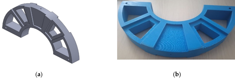
Figure 10. Tool developed for the measurement of the axial component of magnetic flux density: (a) 3D model, (b) printed tool.
