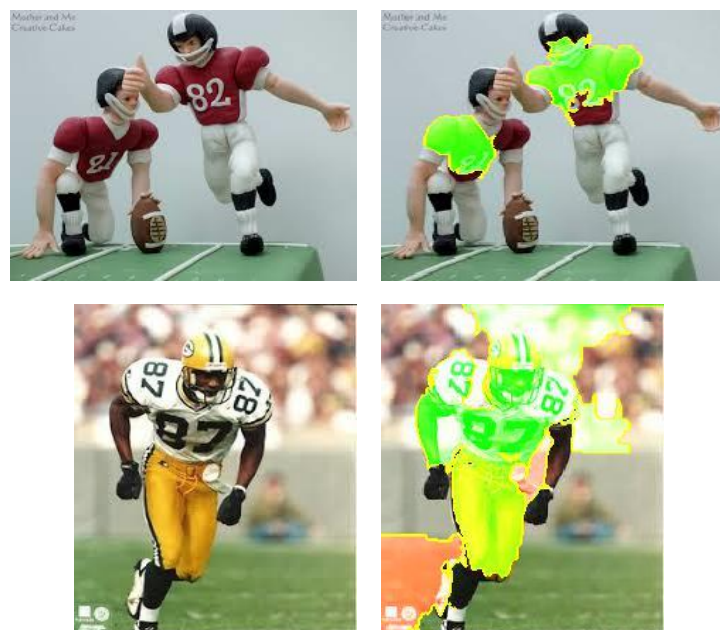
Figure 7. Examples of how LIME explained classifying images as American football. We can see that the equipment, such as helmets, visors, and shoulder pads, of athletes is decisive for classification.
