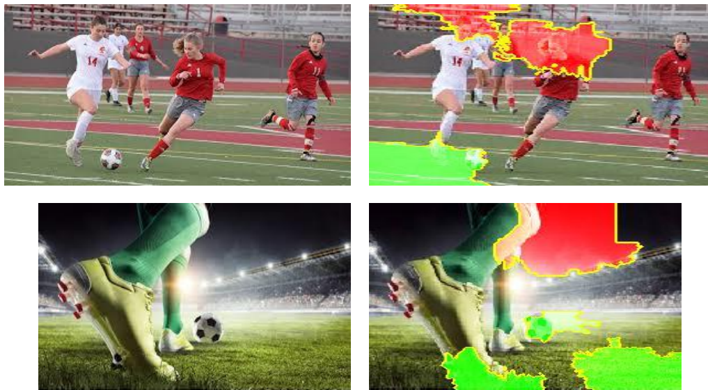
Figure 10. Examples of how LIME explained classifying images as soccer. Here, the shape of the soccer ball or specialties of the soccer shoes are decisive for classification.
