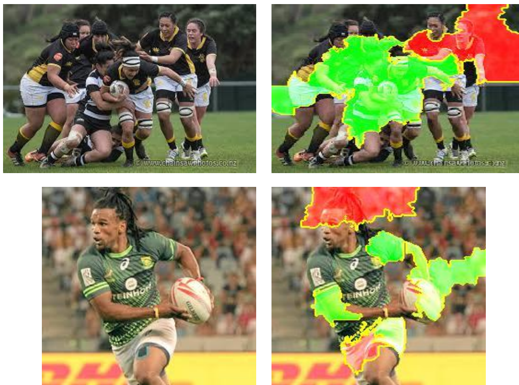
Figure 9. Examples of how LIME explained classifying images as rugby. Here, the packed formation of athletes and the rugby ball are decisive for classification; again, general features of athletes do not contribute to classification.
