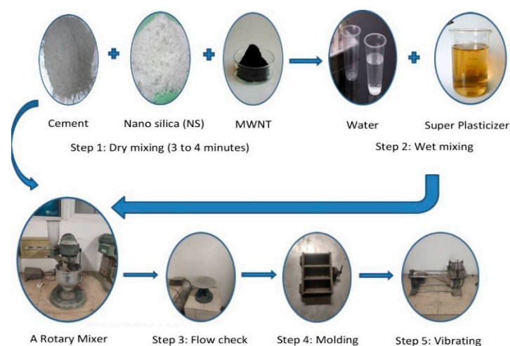
Figure 1. Schematic illustrating the fabrication procedures of the multi-walled carbon nanotubes/nano-silica (MWNT/NS)-incorporated cement composites.
