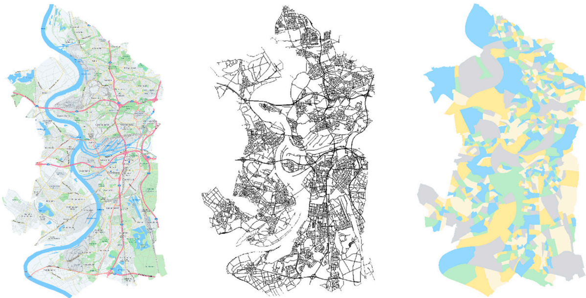
Figure 3. Map (Source: HERE map), road network, and traffic demand partition of city Duisburg.
