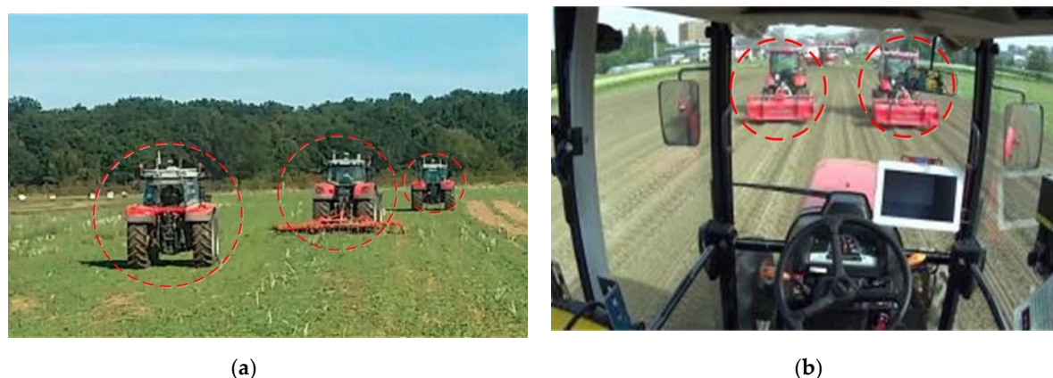
Figure 16. Formations of agricultural multi-robots: (a) the head and tail robots in the formation are used to guide UGVs in I-shape operation. And the robot in the middle of the formation plows with farming tools in the field [44]. (b) Leader-follower method to control the formation in V-shape operation [105]
