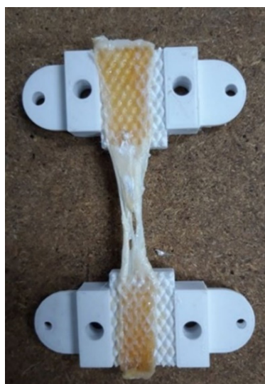
Figure 13. Clamping area and specimen failure.
