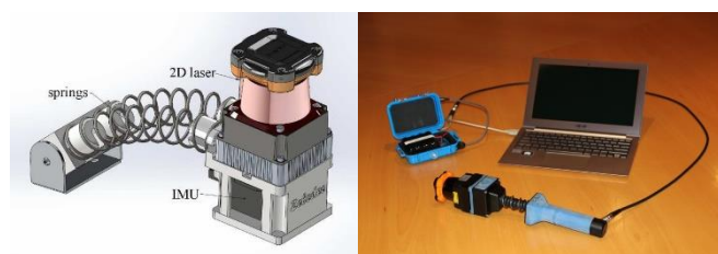
Figure 9. An irregularly moving 2D LiDAR, the movement of the 2D LiDAR is irregular. The prototype in [80,81] is called Zebedee. From this figure we can see the main components of Zebedee—that is, a 2D LiDAR, an IMU, a spring and a handheld pole.
