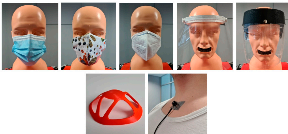
Figure 2. Collection of various face protections used in the experiment ( top )—surgical mask, home-made mask made out of cloth, FFP2 mask, transparent face shields, support under the mask (bracket) and placement of the accelerometer on “suprasternal notch” ( bottom ).
