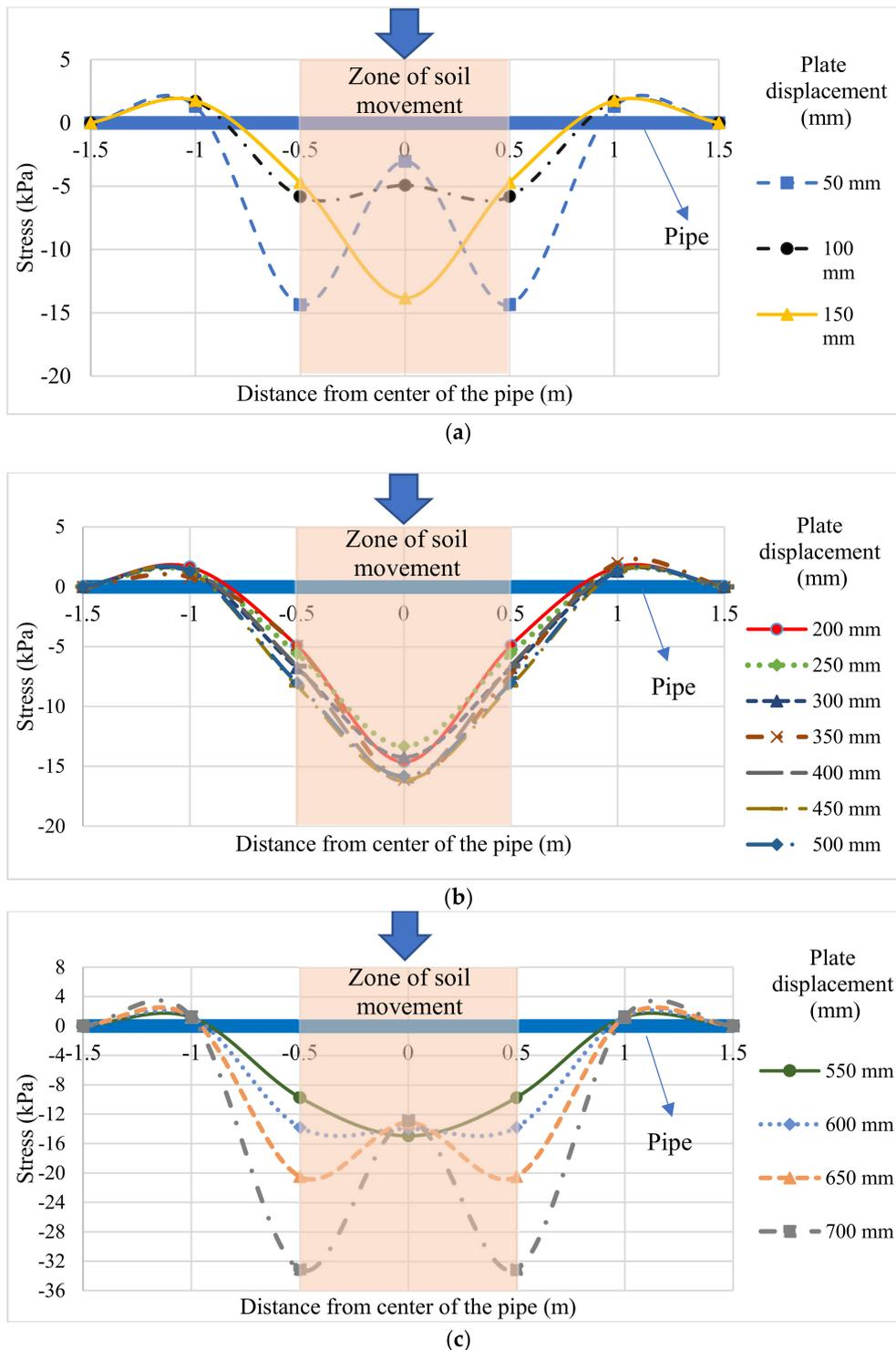
**Figure 6.** (a) Load distribution along the pipe at plate stages from 50 to 150 mm. (b) Load distribution along the pipe at plate stages from 200 to 500 mm. (c) Load distribution along the pipe at plate stages from 550 to 700 mm.
