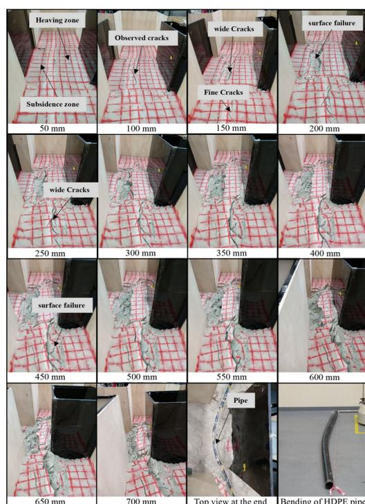
**Figure 8.** Surface displacement of the soil in increasing 50 mm stages by the movement of a plate. Soil cracks are observed at different stages and the pipe bends.
