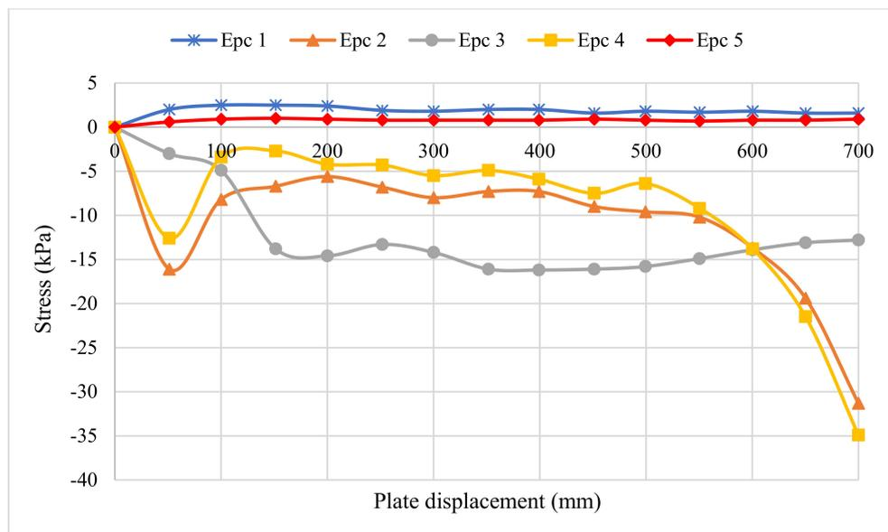
**Figure 5.** Stress values on the buried pipe at different positions.
