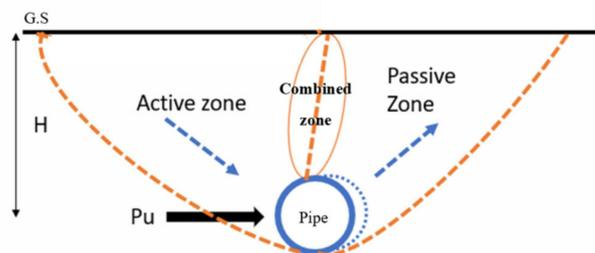
Figure 1. Lateral ground movement on buried pipe (adopted from O'Rourke and Liu [15]).
