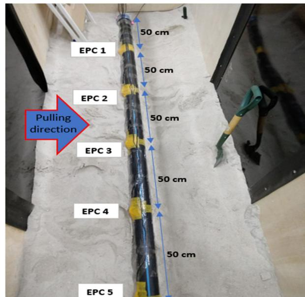
Figure 4. Placement of an HDPE pipe in the middle of the chamber used to assess lateral pipeline–soil interaction in sandy soil.
