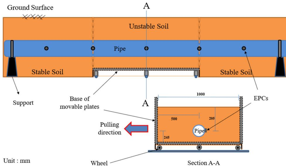
Figure 3. Cross-section of the physical model used to assess lateral pipeline–soil interaction in sandy soil.
