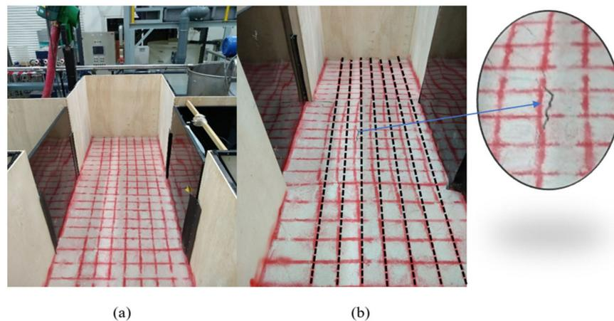
**Figure 7.** Stages of soil displacement (a) initial stage (b) at 50 mm displacement.
