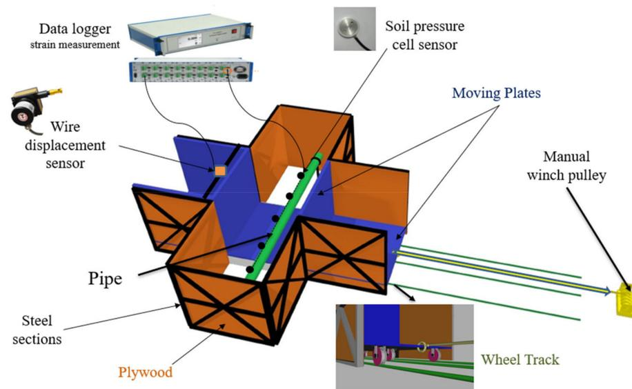
Figure 2. The large-scale model of soil–pipeline interaction.
