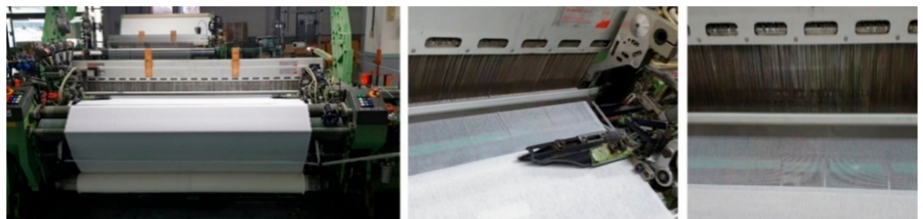
Figure 3. High-density weaving process of shielding fiber.
