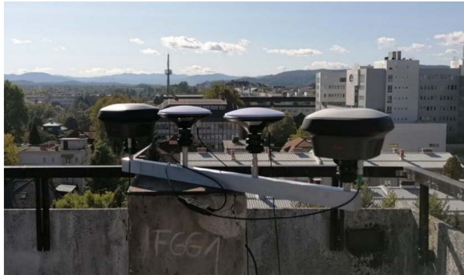
Figure 4. Geodetic and low-cost GNSS devices in the four-point metal arm.
