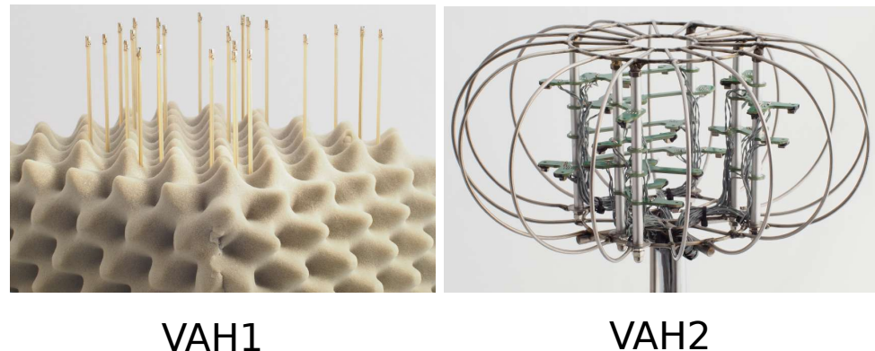
Figure 1. VAHs used in this study. VAH1: a planar microphone array with 24 microphones. VAH2: a 3D microphone array with 31 microphones.
