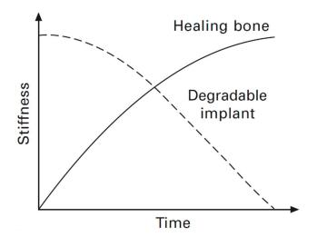
**Figure 3.** A Stiffness–Time inverse relationship between degradable implants and healing bone. Reproduced with permission from Witte, F., et al., Magnesium (Mg) corrosion: a challenging concept for degradable implants; published by Woodhead Publishing, 2011 [60].
