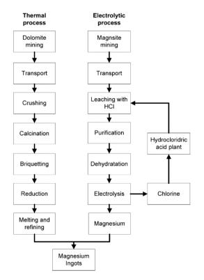
**Figure 1.** Process flowchart of primary magnesium production via a thermal and electrolytic process. Reproduced with permission from Cherubini, F., et al., LCA of magnesium production; published by Elsevier, 2008 [15].
