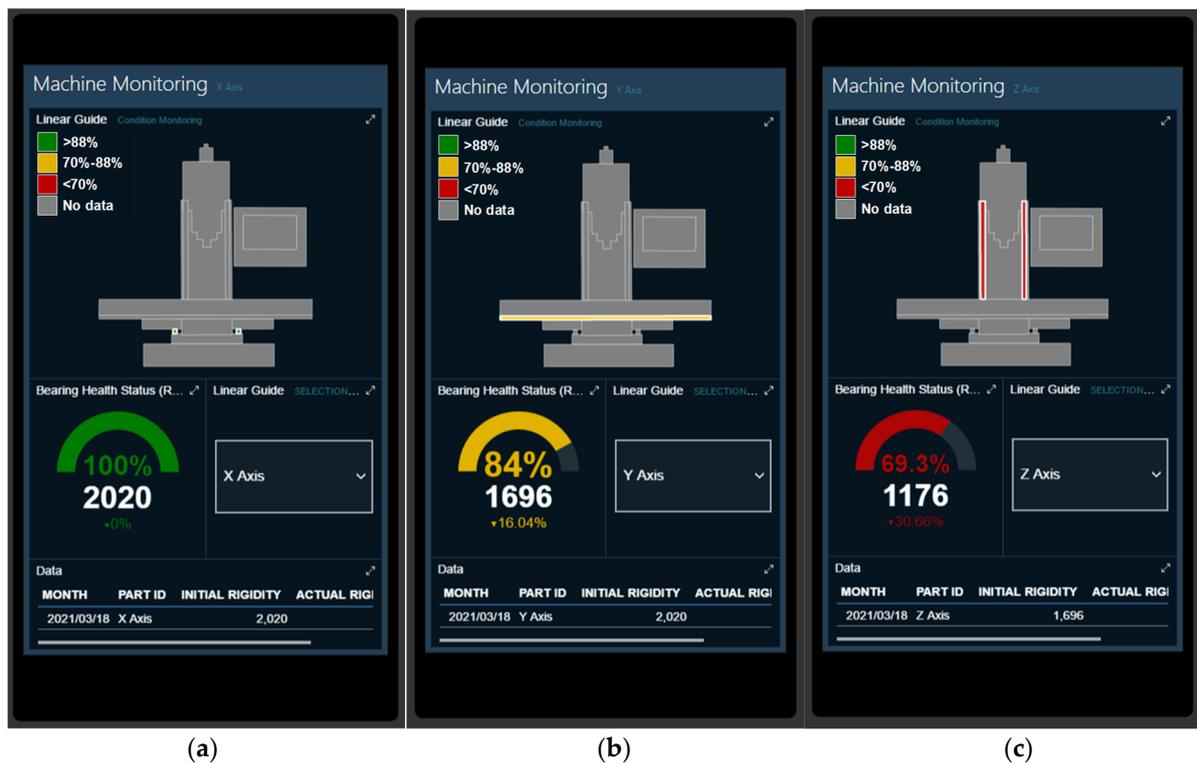
**Figure 17.** Application scenarios of predictive model with graphical user interface for monitoring rigidity decay of feeding mechanisms in milling machine: (a) X axis linear guide; (b) Y axis linear guide; and (c) Z axis linear guide.
