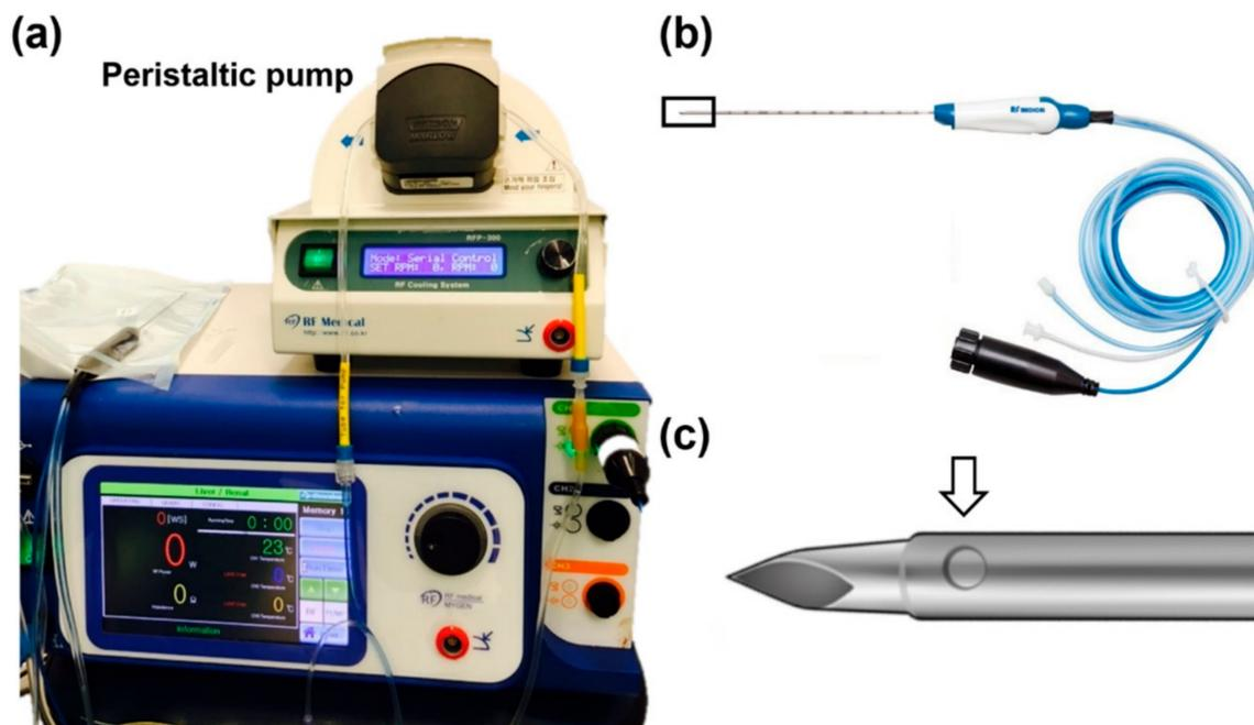
**Figure 2.** The radiofrequency ablation (RFA) system configuration. (a) A three-channel radiofrequency ablation system, which can allow the use of multiple electrodes in either monopolar or bipolar modes. (b) An internally cooled wet electrode with a 2-cm active tip. (c) The magnified image of the DRCWE tip with a side hole (white arrow).
