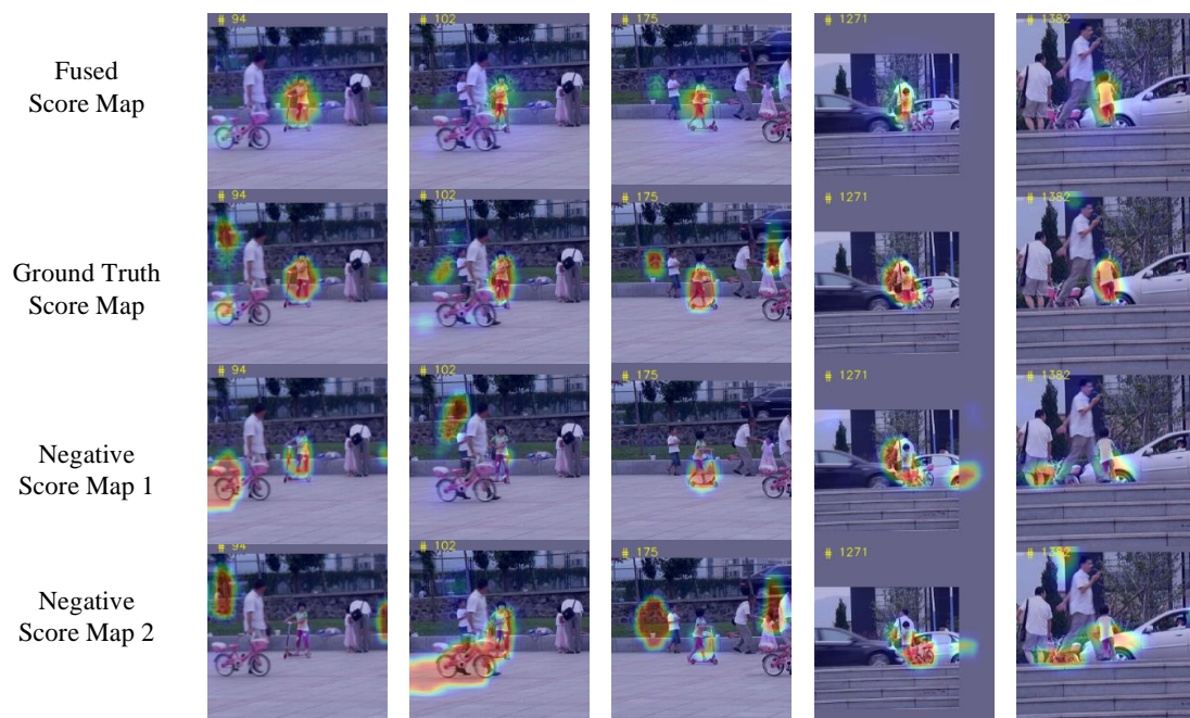
Figure 1. Illustration of our score fusion procedure. The ground truth score map not only responds to the real target but also raises the responses in many other areas where the tracker is easily misled. After implementing fusion, the unrelated responses are sufficiently suppressed.
