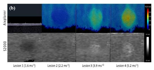
**Figure 3.** Showing: (a) Aixplorer image of a homogenous region of the phantom to illustrate the bands of greater shear wave speed (artefacts) observed. (b) Example elastograms of the lesions contained within the CIRS 049 phantom using the Aixplorer and the S2000. Nominal shear-wave speeds are given below the images.
