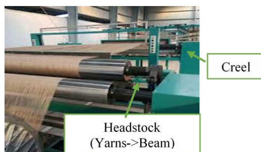
Figure 4. Beaming machine structure.
