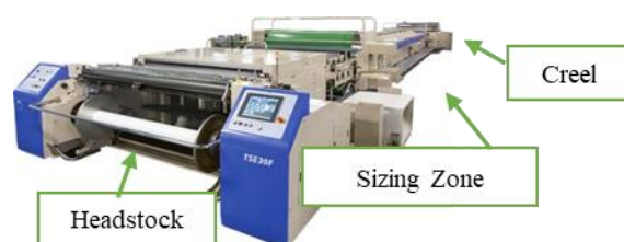
Figure 3. Sizing machine structure.
