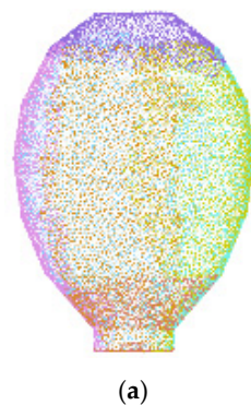
Figure 18. The final 3D reconstruction results: (a) Full registered point cloud; (b) Surface reconstruction model.
