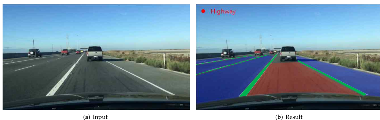
Figure 1. Our goal: Solving drivable area estimation, lane line segmentation, and scene classification through multi-task learning.
