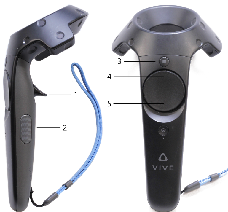
Figure 3. Overview of the Vive Wand wireless controllers. (1) Trigger—create new atoms and bonds; interact with menus. (2) Grip button—move atoms, rotate bonds, or rotate molecule. (3) Menu button—cycle controller between menu and build mode. (4) Touchpad, top quadrant—remove atom or bonds. (5) Touchpad, bottom quadrant—select atoms and bonds for measuring and editing.
