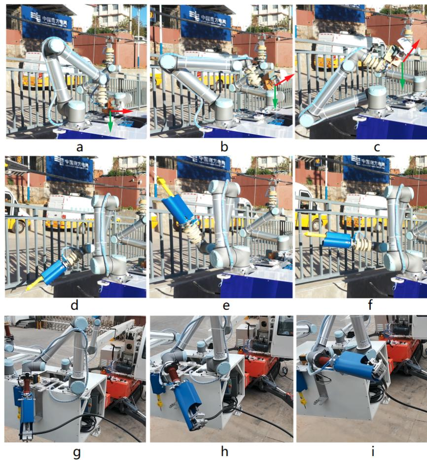
**Figure 23.** The impact of planning algorithms on the task process. (a–c) During the stripping operation, the non-fixed parts should be kept open during the tool removal operation. (d–f) During the movement of the long tool, each joint of the robot is in a proper state of force and the load capacity is improved. (g–i) During the installation of the cable, the robot body maintains the principle cable to prevent entanglement.)
