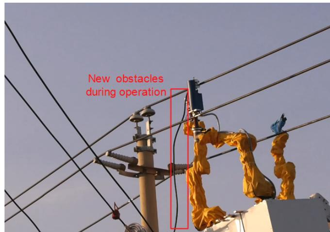
Figure 17. The newly installed drainage wire affects robot movement.
