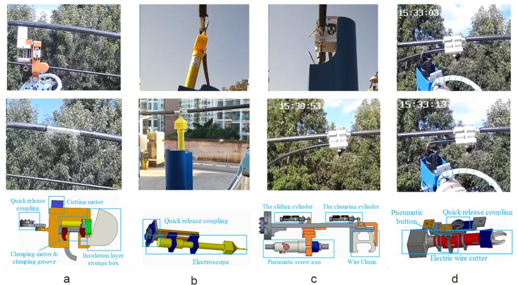
**Figure 2.** Operations of live-line maintenance [27]. ((a) Wire stripping, (b) voltage detection, (c) wire clamp installation, and (d) lead-flow wire cut off).
