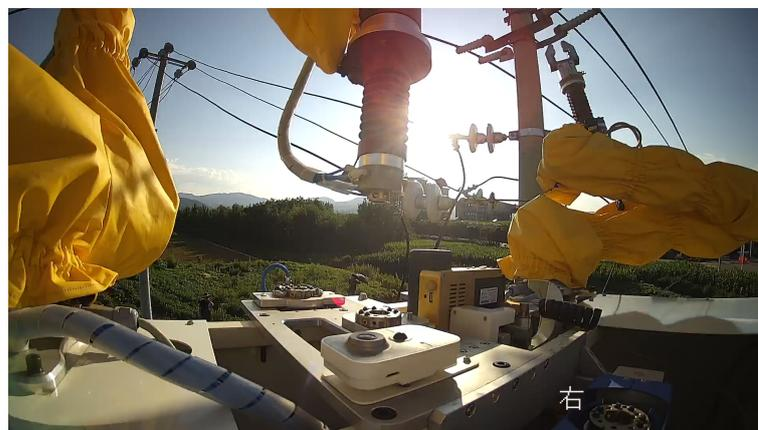
**Figure 4.** Dense tool placement and small space limit robot movement.
