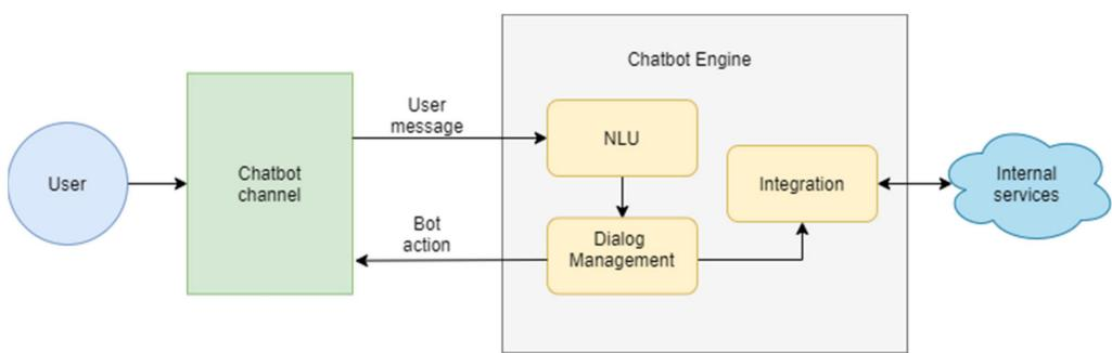
**Figure 3.** Architecture of the module-based chat-bot system.
