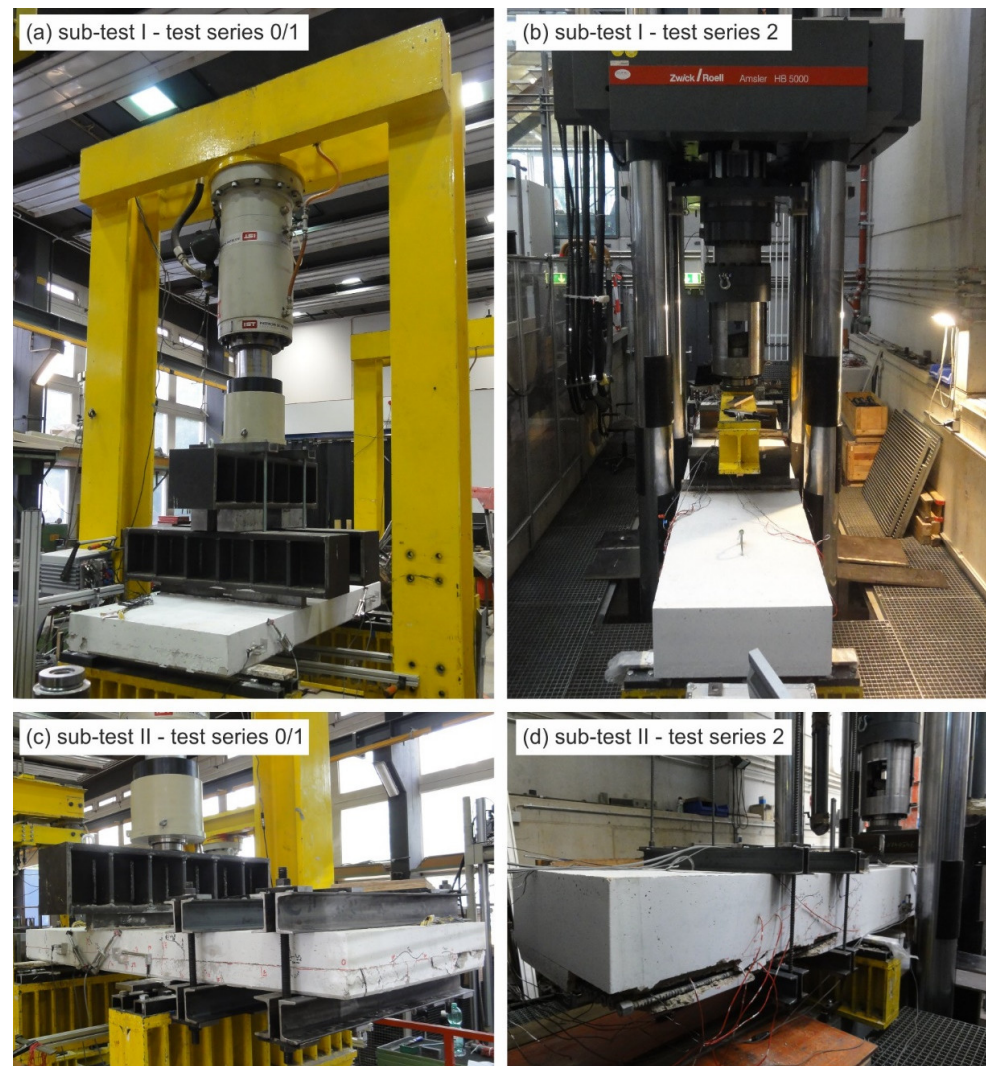
Figure 15. Test setup for fatigue tests: Sub-Test I for Test Series 0/1 (a), Sub-Test I for Test Series 2 (b), Sub-Test II for Test Series 0/1 (c), and Sub-Test II for Test Series 2 (d).
