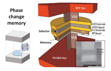
**Figure 3.** 3D schematics and SEM cross section of a GeSbTe (GST) phase change memory integrated with GeSeSbN OTS selector from [71].
