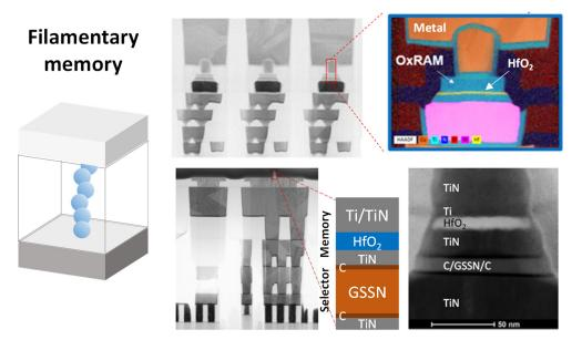
**Figure 2.** TEM cross sections of an HfO<sub>2</sub> based OxRAM integrated in the BEOL of a 28 nm FDSOI technology, from [44] (top) and an OxRAM/OTS device integrated in the BEOL of a 130 nm CMOS process, from [45] (bottom). The OTS (Ovonic Threshold Switch) backend selector is composed of a C/GeSeSbN/C stack.
