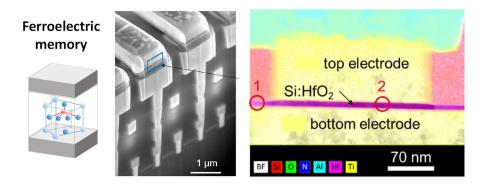
Figure 5. SEM and TEM cross sections of ferroelectric TiN/10 nm Si (1%)-implanted  $HfO_2/TiN$  capacitors integrated between M4 and M5 of a 130 nm CMOS, from [91].
