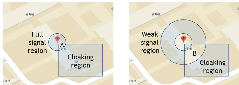
Figure 5. Location attack using AP region with various signal strength.
