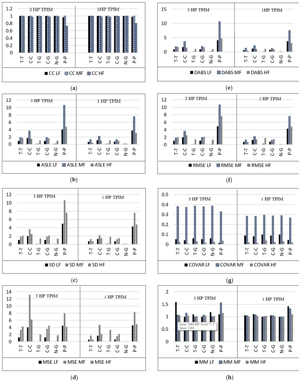
**Figure 8.** The statistical indicators threshold limits for each fault for the 3-HP and 1-HP TPIM (a) CC threshold limits (b) ASLE threshold limits (c) SD threshold limits (d) MSE threshold limits (e) DABS threshold limits (f) RMSE threshold limits (g) COVAR threshold limits (h) threshold limits MM.
