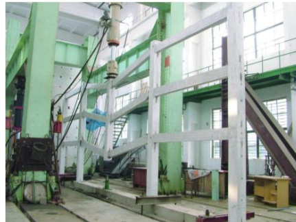
Figure 3. Collapse limit state of model frame.
