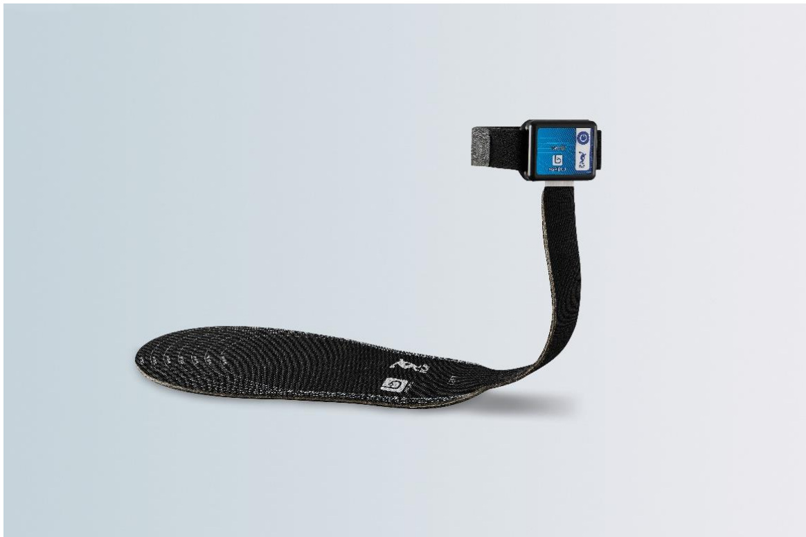
Figure 1. The insole. The device is composed of the insole containing the weight sensors, which is connected with a band to the electronic bio-feedback display. The display is then attached to the patient leg with a Velcro strap.
