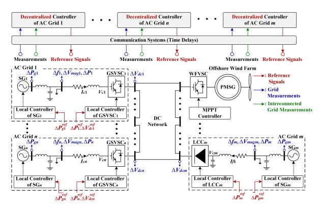
Figure 1. A schematic showing optimal control of hybrid MTDC-linked grids and OWFs.
