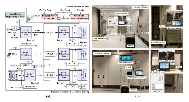
**Figure 13.** (a) A schematic of a new electrical system inside a commercial building and (b) the experimental setup of an MG including a generator emulator, a battery pack, and a load emulator.
