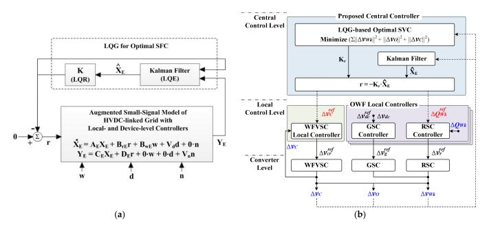
**Figure 2.** Use of an LQG regulator to generate optimal reference signals for the individual local controllers of the HVDC system and the OWFs: (**a**) frequency control and (**b**) voltage control.
