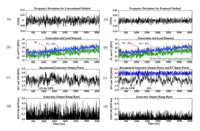
**Figure 15.** Experimental case study results for the (**left**) conventional and (**right**) proposed FR strategies: (**a**) frequency deviations  $\Delta f$ , (**b**) load demands  $P_L$ , dispatchable generation  $P_G$ , and total generation  $P_G + P_{PV}$ , (**c**) variations in generator output power  $\Delta P_G$  and in battery input power  $\Delta P_B$ , and (**d**) dynamic ramping rate of generation  $|d\Delta P_G/dt|$ .
