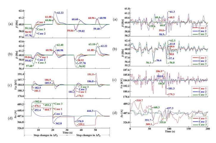
**Figure 4.** Responses to (**left**) step and (**right**) continuous variations in the inverter-side and rectifierside loads and in the OWF power generation when the LQG strategy (Case 1) and conventional PI-based strategies (Cases 2 and 3) are applied: (**a**) inverter-side frequency  $f_i$ , (**b**) rectifier-side frequency  $f_r$ , (**c**) DC-link voltage  $V_{dc}$ , and (**d**) DC current  $I_{dc}$ .
