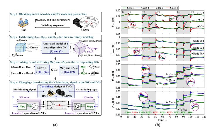
**Figure 12.** (a) A flowchart for implementation of the proposed FVCs and (b) comparisons of  $V_{DG}$ ,  $V_{Load}$ ,  $Q_{DG}$ , and  $P_{DG}$  (from top to bottom) between the new proposed VR strategy (Cases 1 and 2) and conventional VR strategies (Cases 3 and 4) for NR-aided load restoration.
