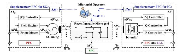
Figure 9. Schematic of a proposed FR strategy for an islanded, reconfigurable MG.
