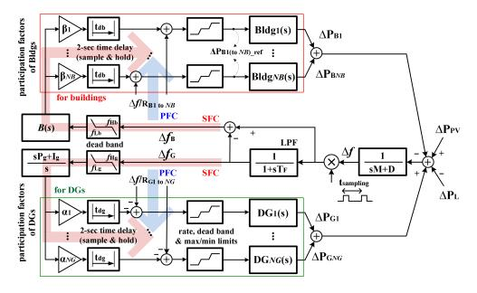
Figure 14. A block diagram of the ancillary service provision by buildings including EV batteries.
