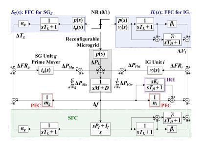
**Figure 10.** A small-signal model of an islanded reconfigurable MG with supplementary FFCs showing the feedback loops for the inertia response emulation and primary and secondary frequency control.
