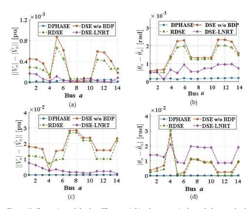
**Figure 17.** Comparison of absolute SE errors: (**a**,**b**) voltage magnitudes and phase angles for the BD in the SCADA measurements and (**c**,**d**) voltage magnitudes and phase angles for the BD in the PMU measurements.
