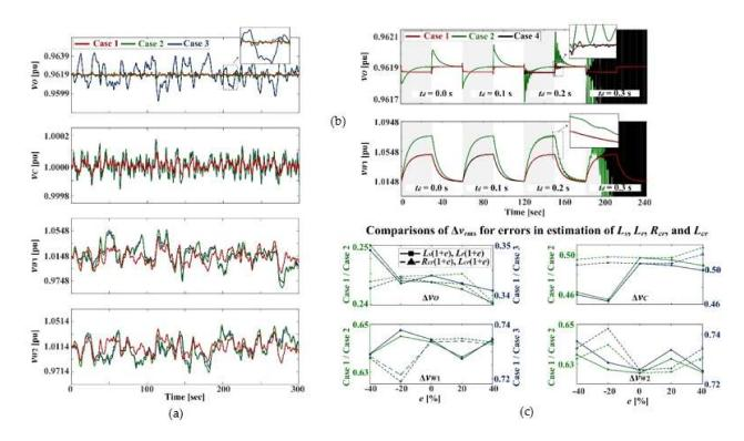
**Figure 5.** Voltage responses to (**a**) continuous variations in OWF power generation, (**b**) a communication time delay  $t_d$ , and, (**c**) uncertainties in inductance and resistance parameters when a novel SVC strategy (Case 1) and conventional PI- and MPC-based SVC strategies (Cases 2 and 3) were applied. In (**a**),  $v_O$  and  $v_C$  are the POC and PCC voltages, respectively, and  $v_{W1}$  and  $v_{W2}$  are the OWF terminal voltages.
