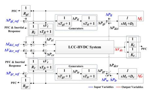
**Figure 3.** A small-signal model of HVDC-linked grids considering the dynamics of the DC link, the converters, and the inner feedback loops.
