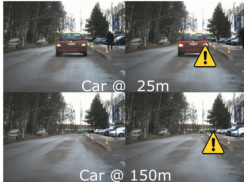
Figure 8. Range test with preprocessing at 25 m and 150 m, warning triangle indicating detected brake lights.
