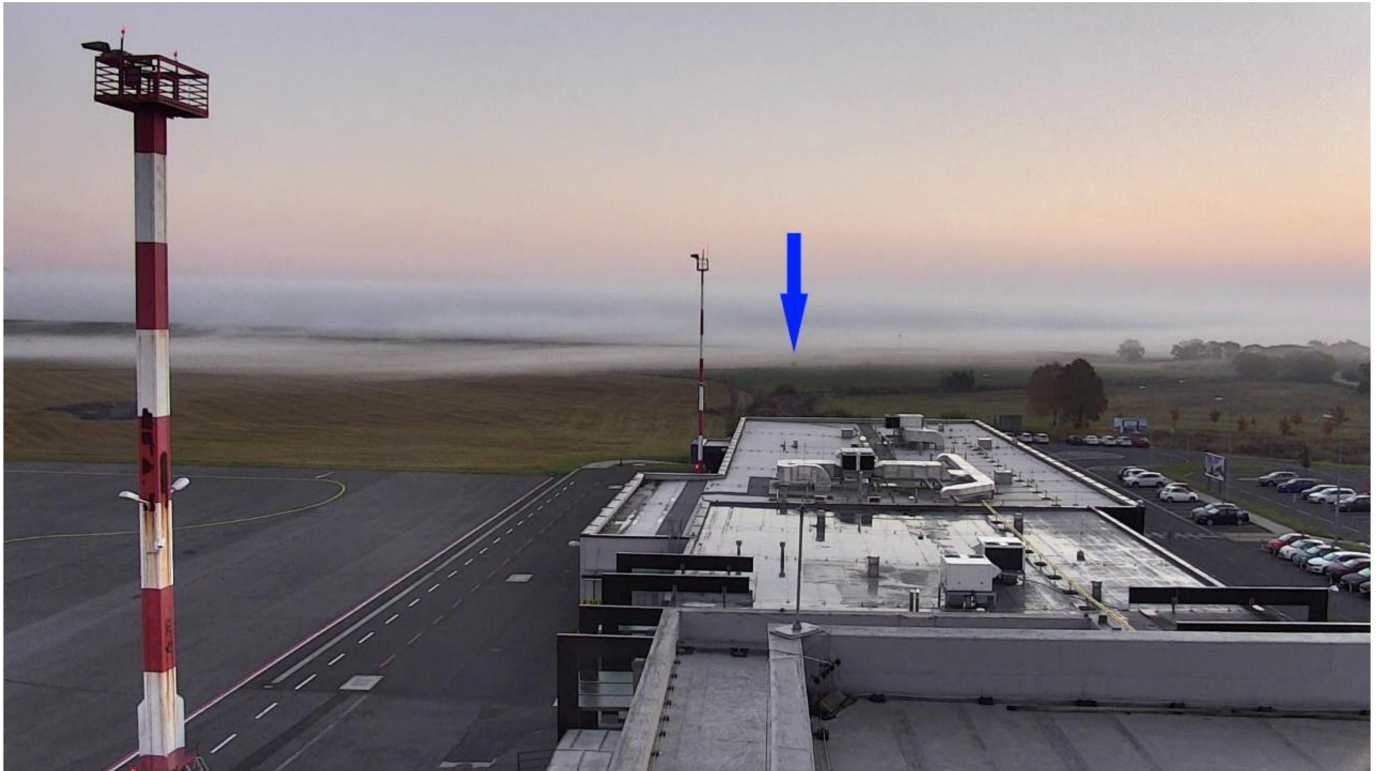
Figure 2. An example to illustrate the drawbacks of point measurements of visibility. Here, the visibility meter (indicated by the blue arrow) gets hidden in a fog patch and reports decreased visibility, but the overall prevailing visibility is higher.
