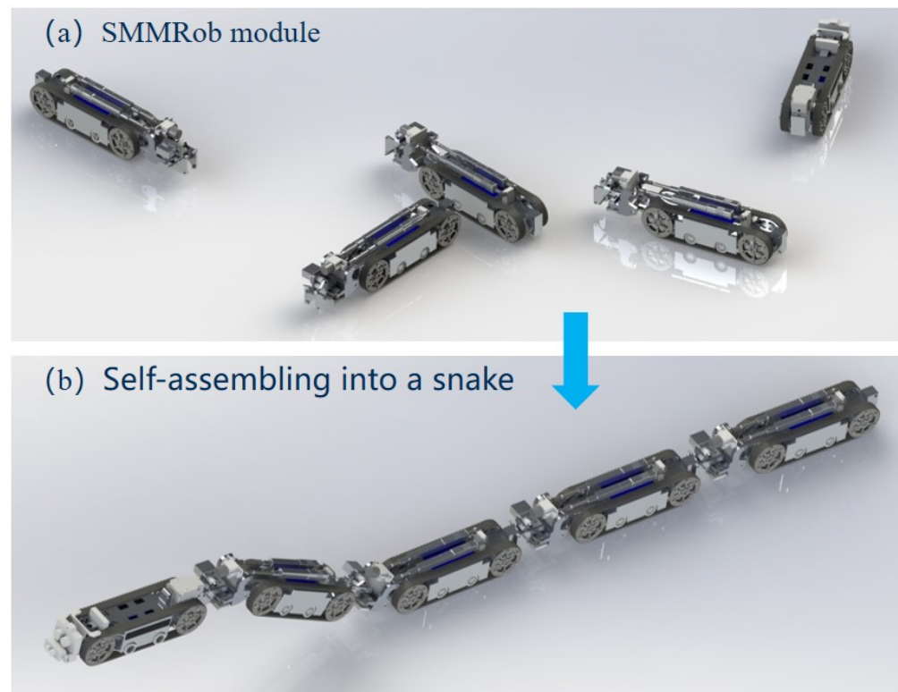
Figure 2. A self-assembling mobile modular robot system consisting of a group of self-contained robot modules and modules with a different function forming the head. (a) Each homogeneous SMMRob module with a different payload can move, sense, manipulate, and dock individually. (b) The robot modules can connect together to form a snake-like high-level system that can move on tracks with joints.
