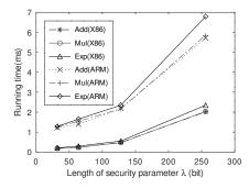
**Figure 2.** The running time comparison of additive, multiplicative and exponential arithmetic operations of LPCP on ARM and X86 architecture.
