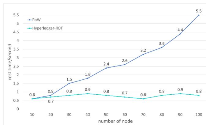
Figure 25. Consensus speed comparison between Hyperledger-IIoT and PoW(Proof of Work).
