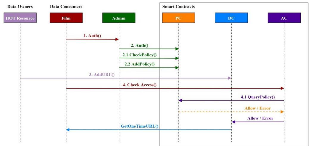
Figure 10. Access control sequence diagram.
