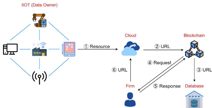
Figure 11. Hyperledger-IIoT Architecture.
