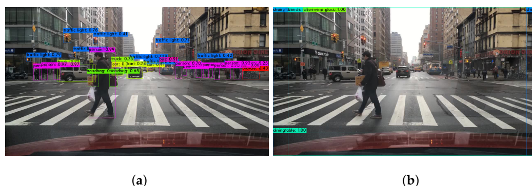
Figure 1. Example of a single-bit error impact in an object detection application based on CNNs. (a) Error-free or single-bit error (bit 705) inference; (b) Single-bit error (bit 734) inference.
