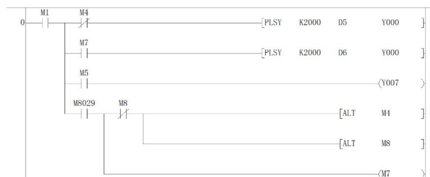
Figure 14. PLC program line diagram of initializing and changing center distance of the cutter.
