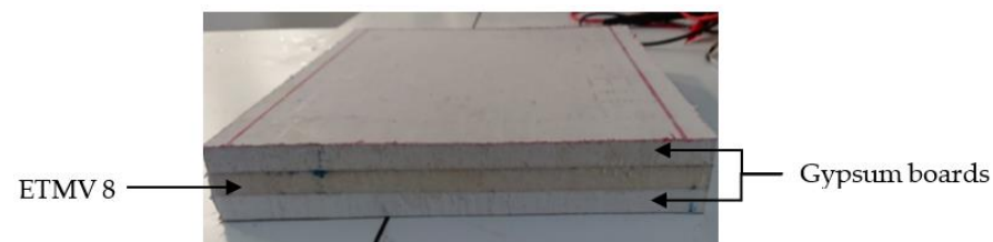
Figure 3. View of the ETMV8 Sample-gypsum board used for experimental tests.
